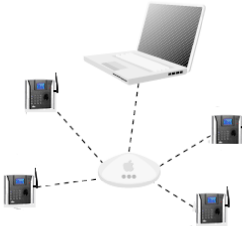
Ad-hoc (peer-to-peer) wireless network
