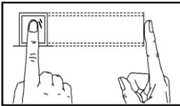
The finger is flat to the surface and centered in fingered guide.
